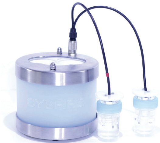
Figure 4: Differential impedance spectrometer on MU-EIS system with temperature stabilization of samples and electronic components.
