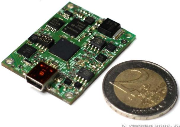
Fig. 2. One module of the measuring system MU2.0, manufactured by *Cybertronica Research*.
