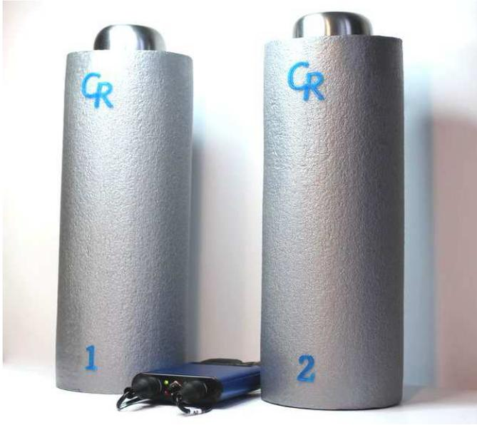
Fig. 3. Prototype of precision differential USB  $pH$ -meter based on MU2.0.
