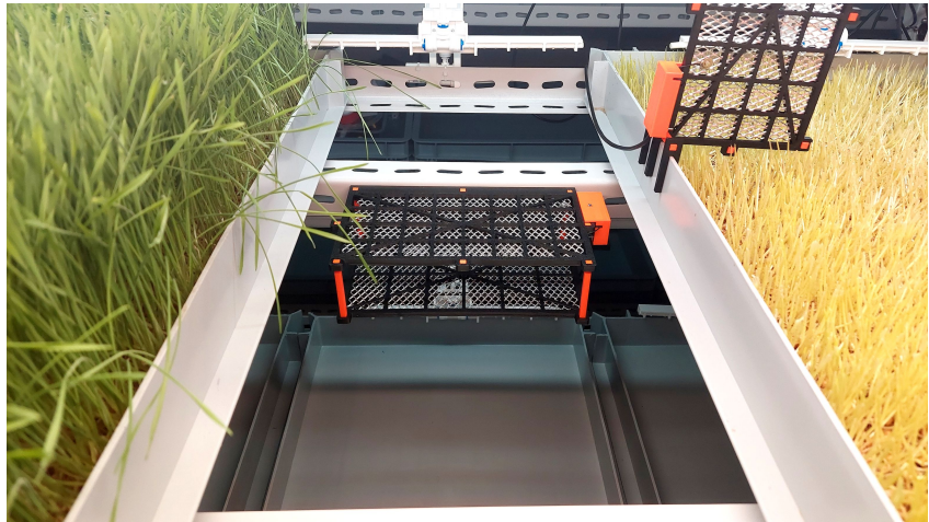
Figure 17: Root biomass and irrigation sensor placed below the growth containers.
