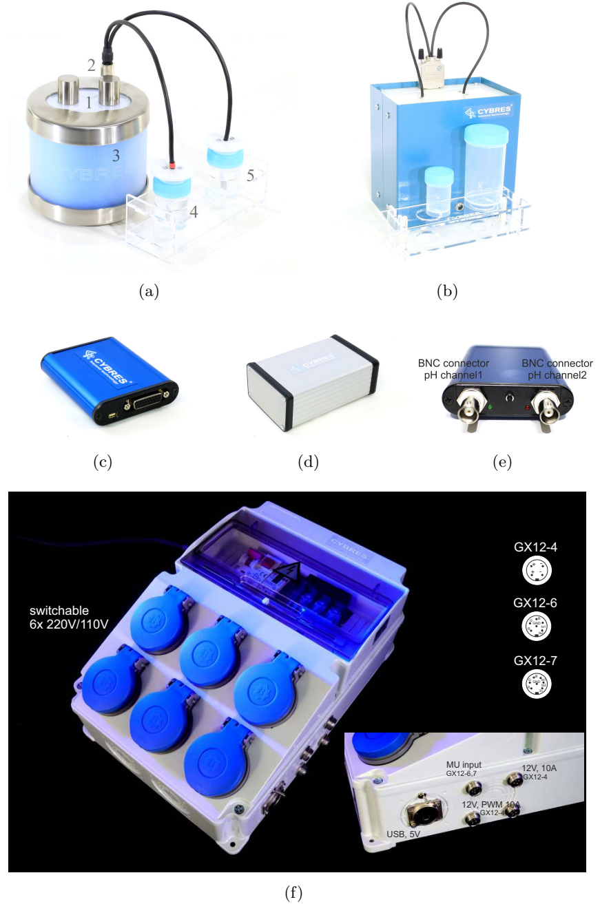
Figure 9: (a) the embedded version of MU EIS differential impedance spectrometer; (1) – measurement cell with two channels (closed by lids on the image), (2) – connector for two electrodes; (3) – hull with RGB LEDs, electronics and additional sensors; (4) – electrode, the channel 1 (with red mark); (5) – electrode, the channel 2; (b) the embedded version of biosensor (for comparison – 15ml and 100ml containers); (c,d) the measuring unit (MU) MU3 and MU3T (with enhanced termostabilization); (e) the MU for differential pH measurements; (f) the power management module with 6 switchable outputs.
