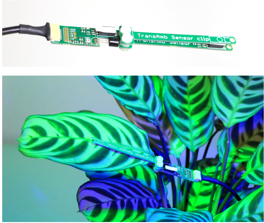
Figure 10: The transAmb stick – Leaf transpiration sensor with environmental sensors (air humidity, light intensity, air temperature).
