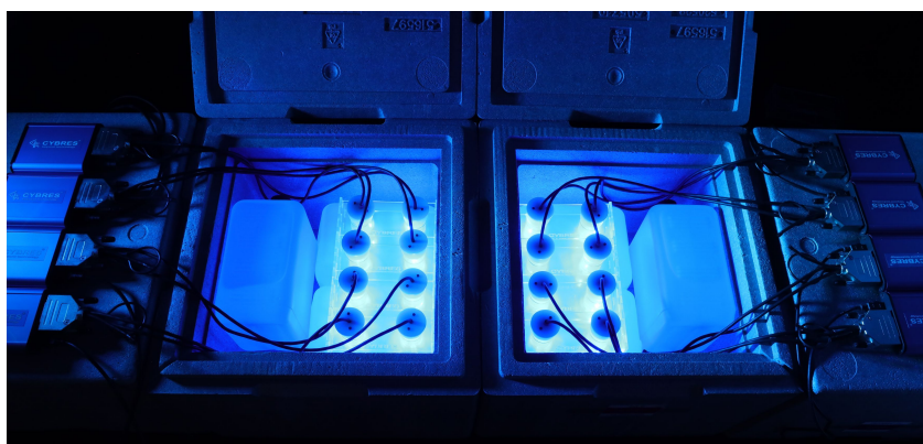
Figure 8: MU systems (MU3 units + open EIS electrodes) used for electrochemical analysis of fluid samples.
