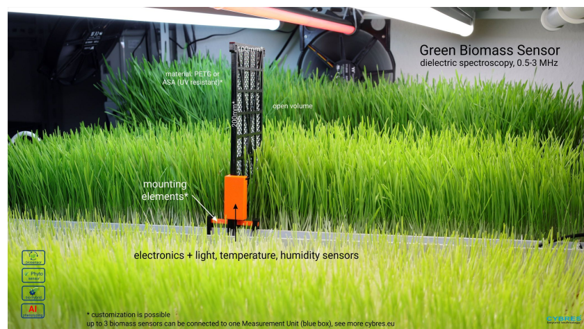
Figure 6: Green biomass sensor (open volume measurement) in indoor farming environment for monitoring of water distribution by root and green biomass, and optimization of water flow.
