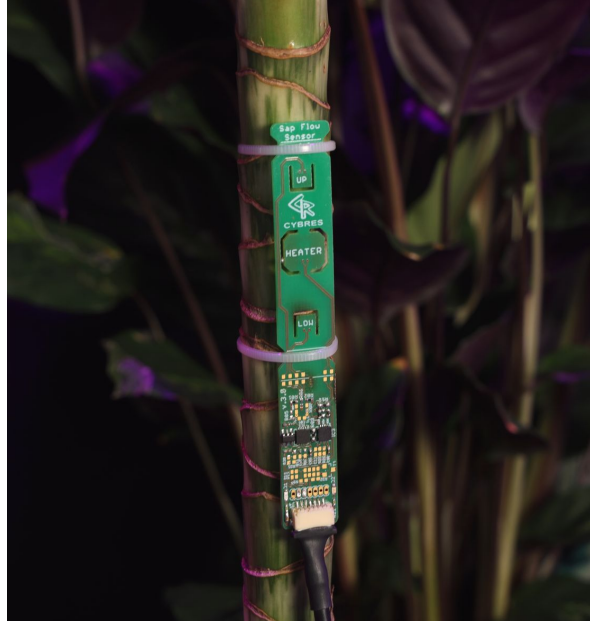
Figure 12: Heat-based sap flow sensor with two upflow and downflow temperature sensors and a heater between them.
