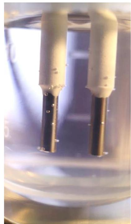
Figure 1. Building of gas bubbles on electrodes.
